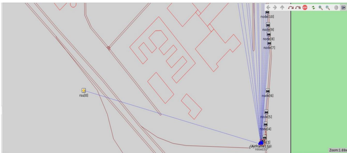
Figure 3. RSU receives signals from node 0 via V2I communication.
